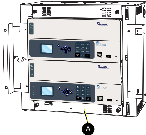
ERn enclosure with [A] an ERn-RPS Mk2 installed in the bottom option slot.
